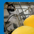
Expansion of the EPS foam is done by using heat, and requires experienced operators.
