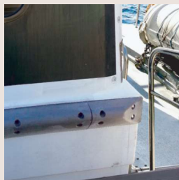
The modules are flexible and can be shaped along the profiles of different boats.
